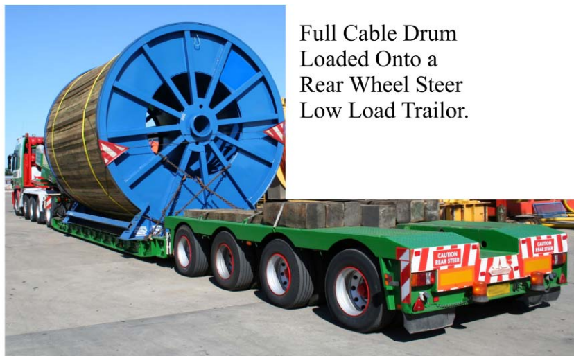
Figure 8 Cable Drum Load Transversely onto a Trailer
